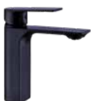
RB.45.MB Basin Faucet Brass body 35 mm cartridge with 2 inox flex 60 cm
